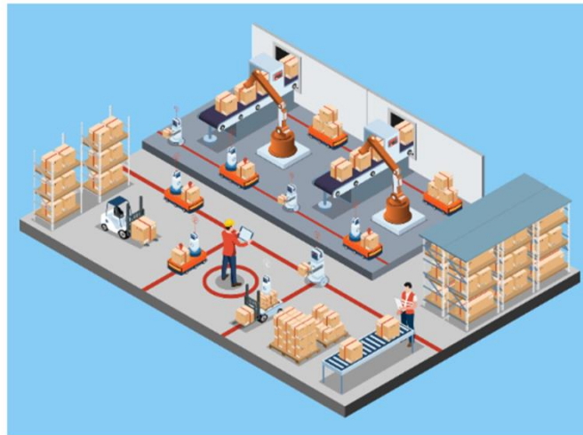
Figure 1: Three-dimensional schematic display of AMR and AS/RS integration in a smart logistics center (Source: Shutterstock / Adapted under an open academic license).
